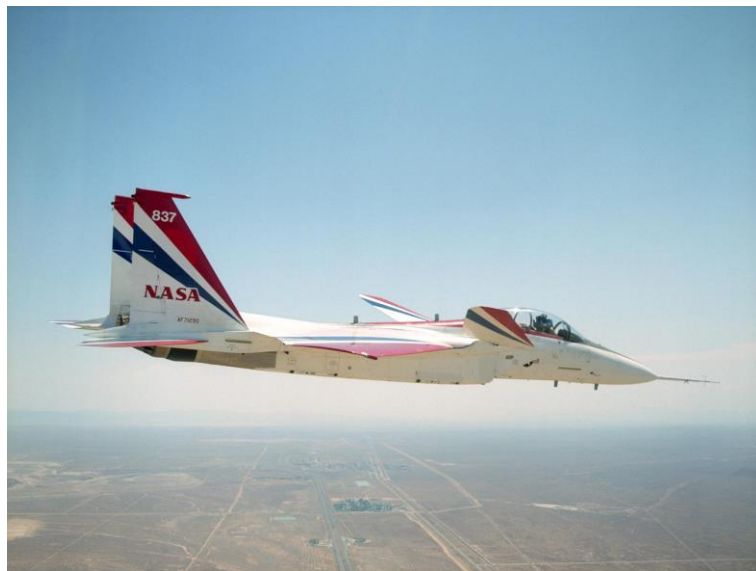
Figure 2 ~ The NASA NF-15B on an Intelligent Flight Control System Mission
