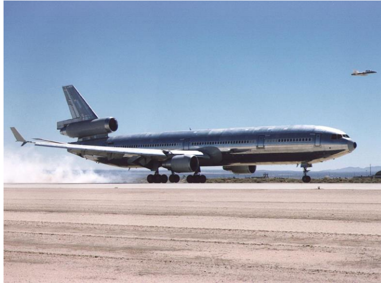
Figure 1 ~ PCA MD-11 landing at Dryden under Propulsion Control, 1995-08-29
